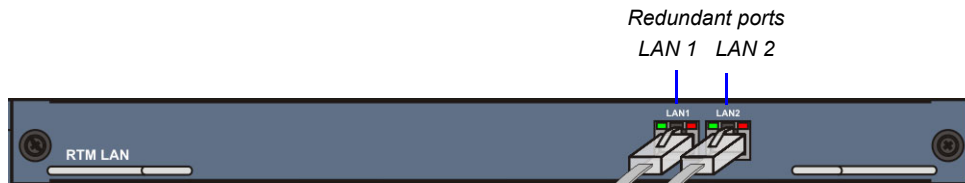
Figure 16-2 RealPresence Collaboration Server (RMX) 2000/RealPresence Collaboration Server (RMX) 4000 RTM LAN Card on Rear Panel
